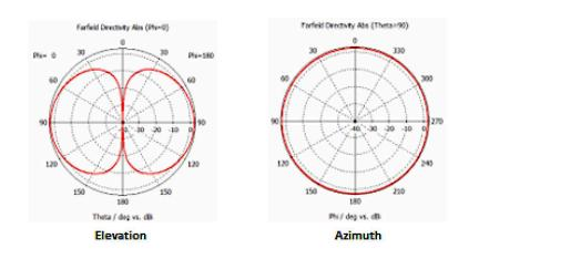
The EMR150FC2 is a vertical base station antenna covering the 144-174 MHz band. This antenna offers a stable radiation pattern across the entire band. The antenna is enclosed in a heavy-duty fiberglass radome and has a fixed N type female connector.
